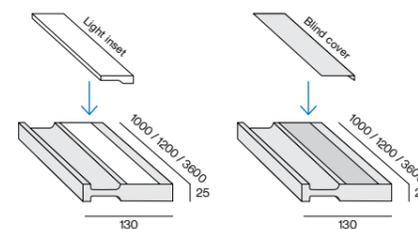
Mounting rail module with light inset
