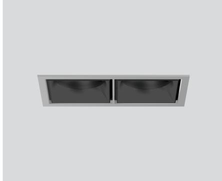
black , RAL9005 1 Mounting set silver-grey front IP40, back IP20 3880 lm **LED** 3000 K CRI ≥ 90 L80 / 50000 h initial MacAdam ≤ 2 SDCM  $R_g$ : 100 ,  $R_f$ : 91 ,  $R_{\{1-15\}}$ : 88 MR 0.59 MDER 0.53 Optical
