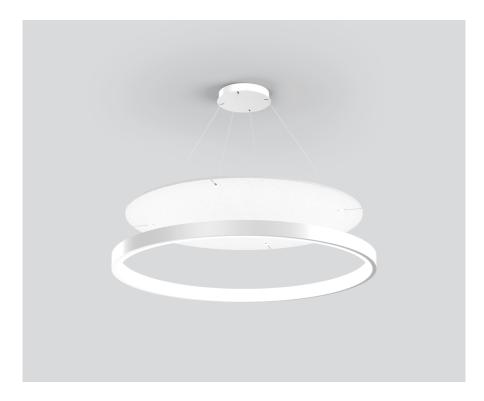
Acoustic element made of high quality, self-supporting PET felt with sound absorbing properties, consisting of 50% recycled PET; round design; high quality visual and tactile surface, white; colour may deviate; for mounting on the INO circle suspended cable suspensions, above the luminaire; subsequent attachment possible;
