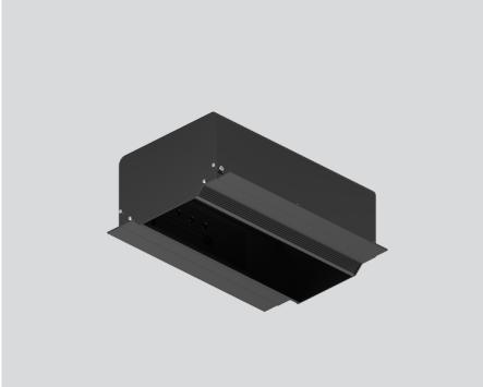
Installation housing in pressed steel sheet with rectangular cut-out; with wrap around edge; suitable for ceiling thickness of 12.5 mm; 6 non-reversible plug and play connector sockets for power supply to the spotlights; spotlight can be installed and moved without tools by means of magnetic holders; hot plug protection; surface jet black powder coated; degree of protection IP20; PC1 220-240V; incl. DALI-2 converter; all spotlights
