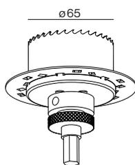
MOVE IN 32 cut out tool for plasterboards
