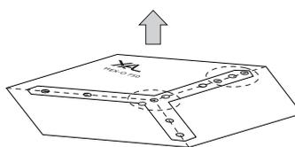
DRILL THE HOLES FOR SUSPENDED SINGLE MOUNTING
